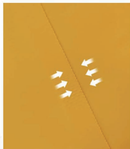
High frequency voltage fusion welding process
